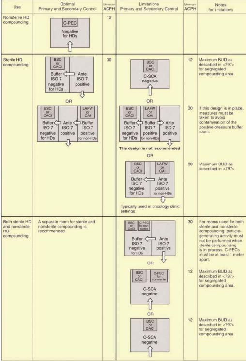
a The arrows indicate direction of airflow.
